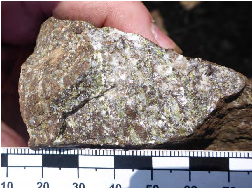
Monazite crystals (green) within ferroan dolomite carbonatite at Kangankunde Sunbird Kuchawe Hotel
